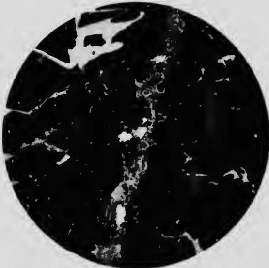
Microphotograph illustrating the occurrence of diamond in veinlets traversing chromite. Magnified 25 diameters.
